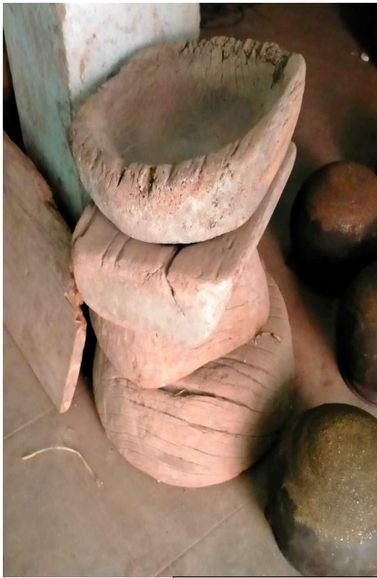
Figure 6 Athaws Used for Preparing Various Types of Traditional Clay Items
