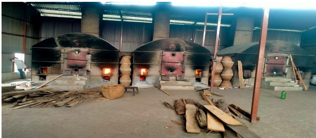
Baking of Clay Items in a Kiln under the Rooftop
