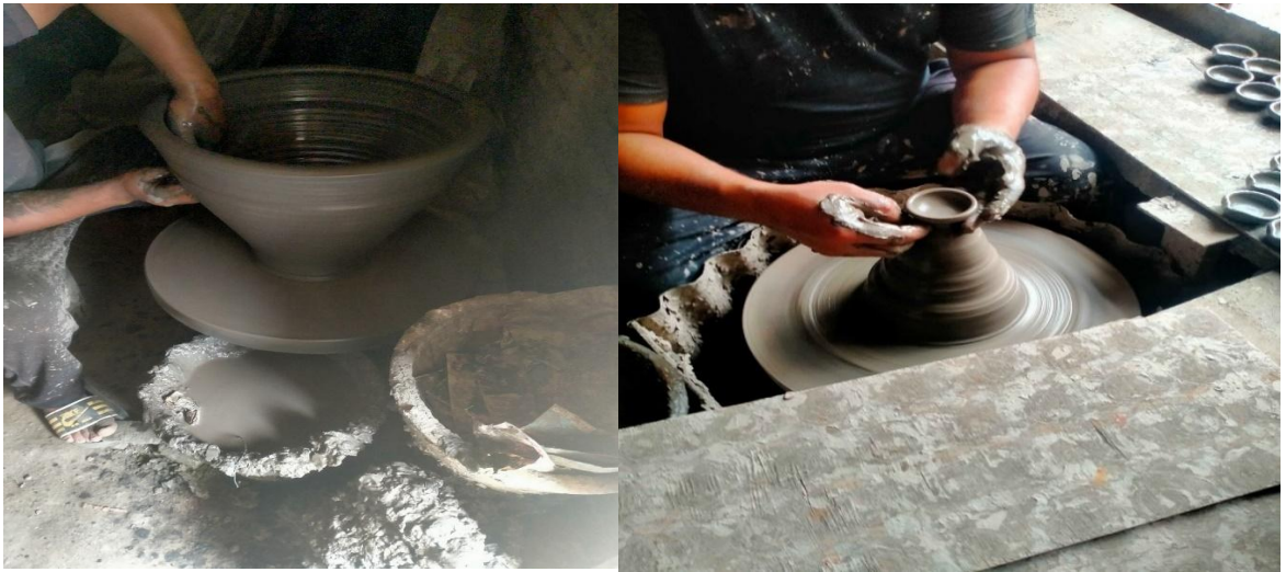
Production of Clay Items in a Motor-Driven Electric Wheel
